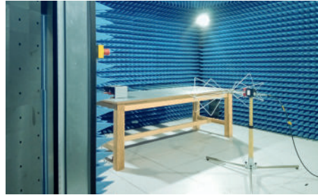
EMC measuring chamber
